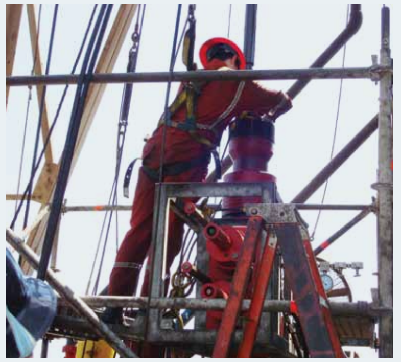
Perforation and stimulation work under way on board the drilling rig, Noble Kenneth Delaney.
